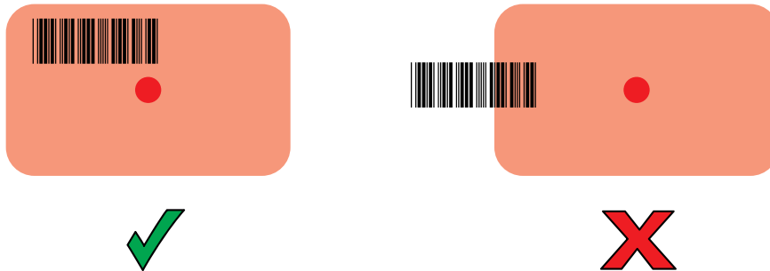
Figure 100 DS3678-SR Pick List Mode with Multiple Barcodes in Aiming Pattern
