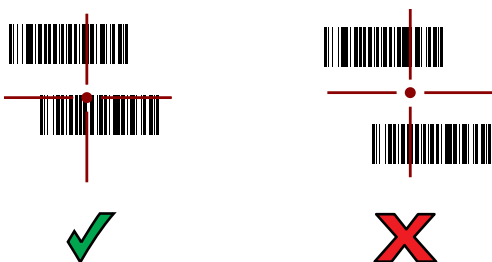
Figure 97 RS507/RS507X Pick List Mode with Multiple Barcodes in Aiming Pattern
