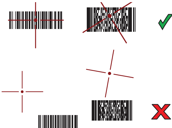
Figure 97 RS507/RS507X Pick List Mode with Multiple Barcodes in Aiming Pattern
